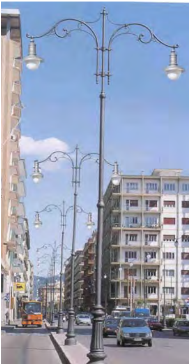
OPTION 4 Type: SB / Double Head 30' Pole Lamp: 250W HPS / 100W Metal Halide
