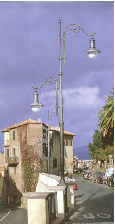
OPTION 4 Type: SC-1 / Double Head 22' Pole Lamp: 100W Metal Halide
